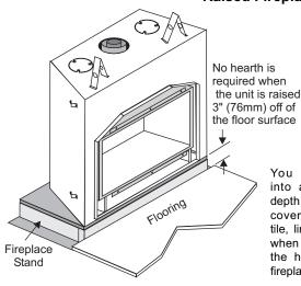
You must take into account the depth of the floor covering (carpet, tile, linoleum, etc.) when determining the height of the fireplace stand.
